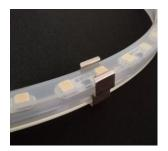
4. Ensure the curve of the WAKO HEBI Curve Light Strip is not less than radius of 85mm.
