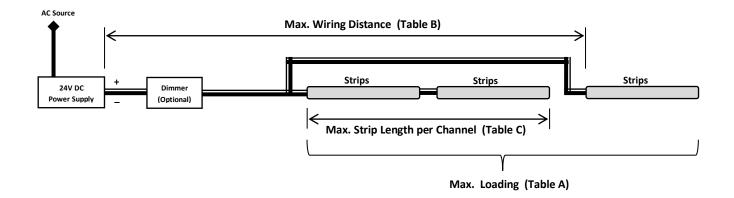
NOTE: MAKE SURE NOT TO EXCEED THE MAXIMUM LIMITS DURING INSTALLATION.
